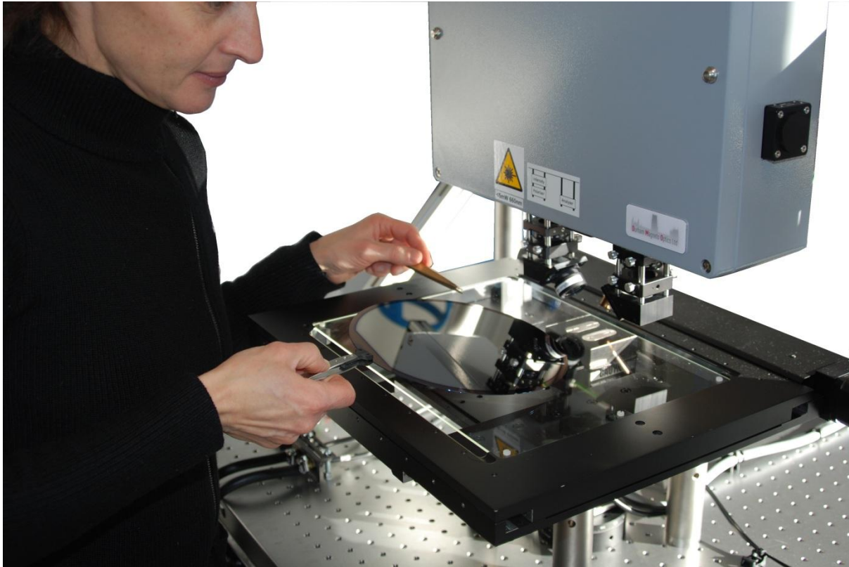
Loading a 200mm wafer into the NanoMOKE3 Wafer Mapper
