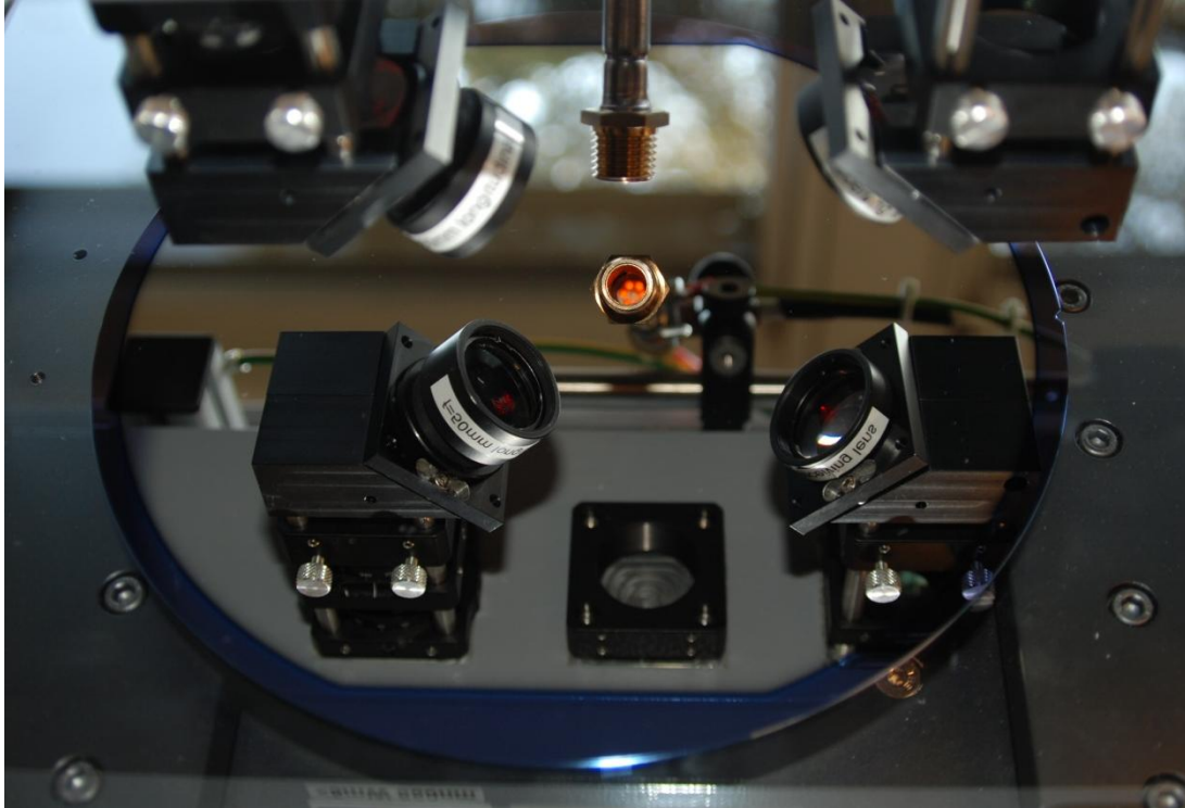
Making elevated temperature measurements under hot gas flow. The picture shows the gas heater pipe with its red-hot filament visible in its reflection in a 200mm wafer.
